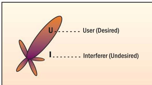
Figure 6. Illustration of a Beam-and-Null Pattern
