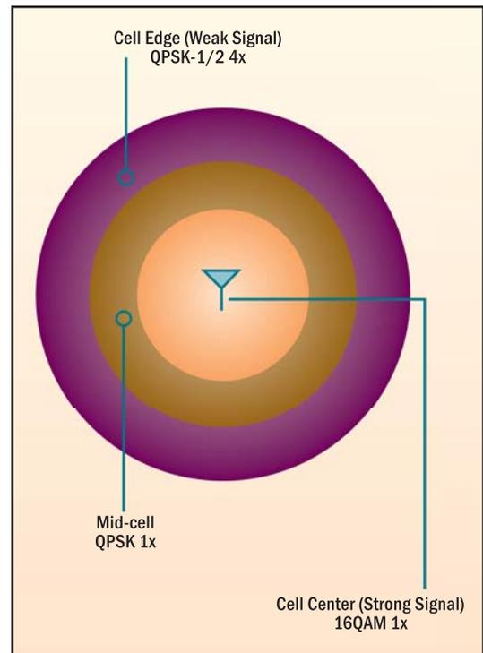
**Figure 1. Illustration of the Use of Modulation Methods (Mod Classes)**
