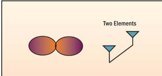
Figure 4. Two-Element Radiation Pattern
