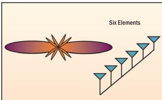
Figure 5. Six-Element Radiation Pattern
