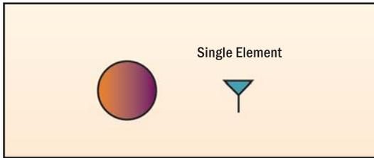
Figure 3. Single-Element Radiation Pattern
