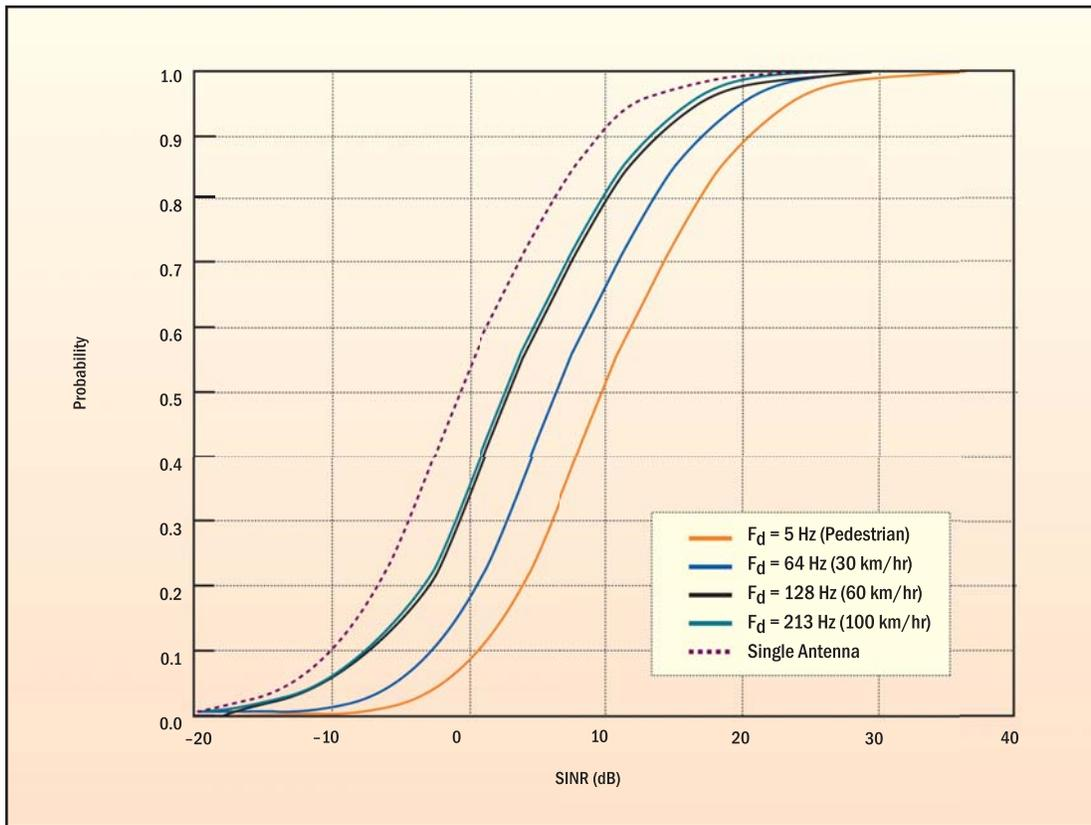
Figure 8. Four-Antenna Mobile WiMAX Simulation Results
