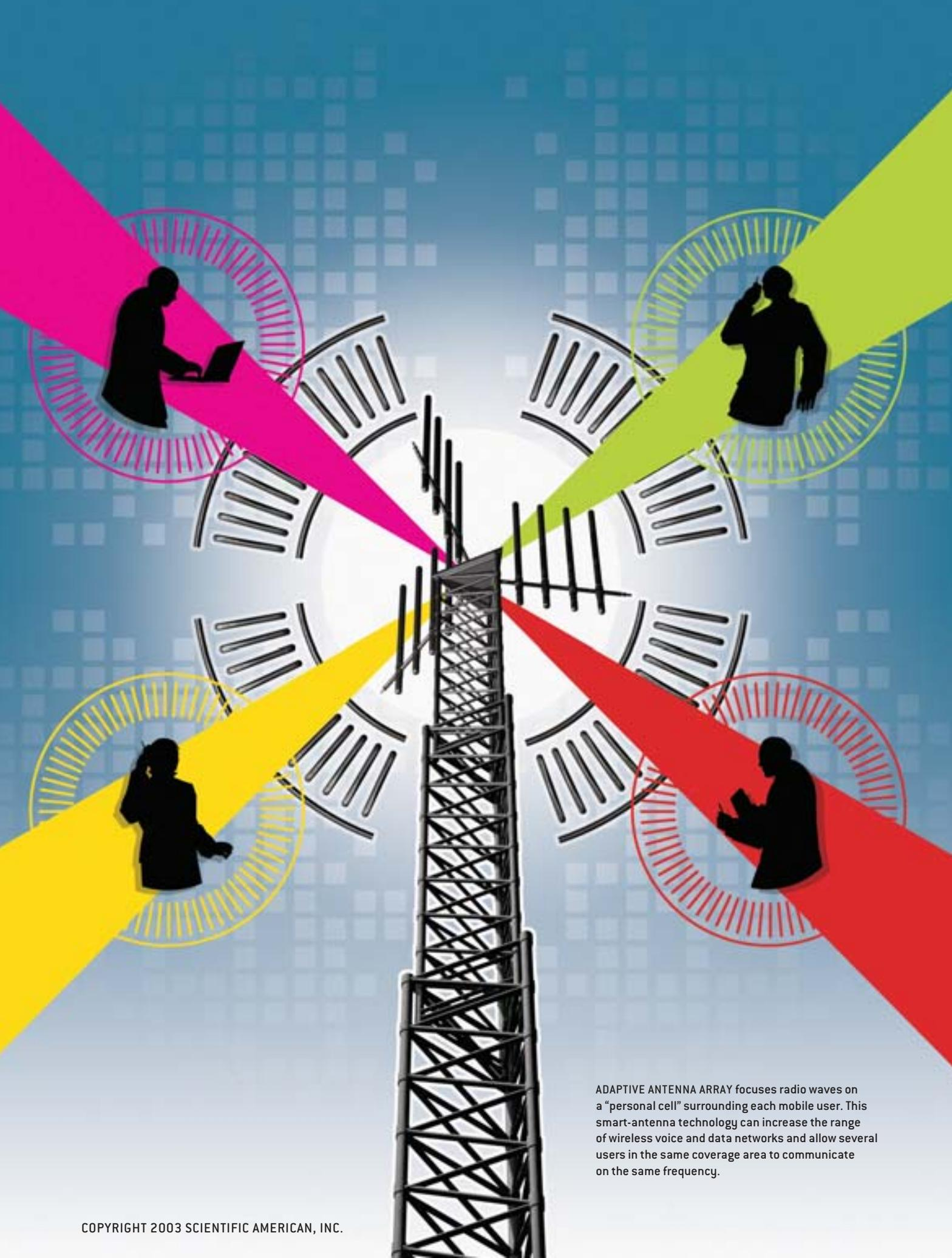
ADAPTIVE ANTENNA ARRAY focuses radio waves on a "personal cell" surrounding each mobile user. This smart-antenna technology can increase the range of wireless voice and data networks and allow several users in the same coverage area to communicate on the same frequency.
